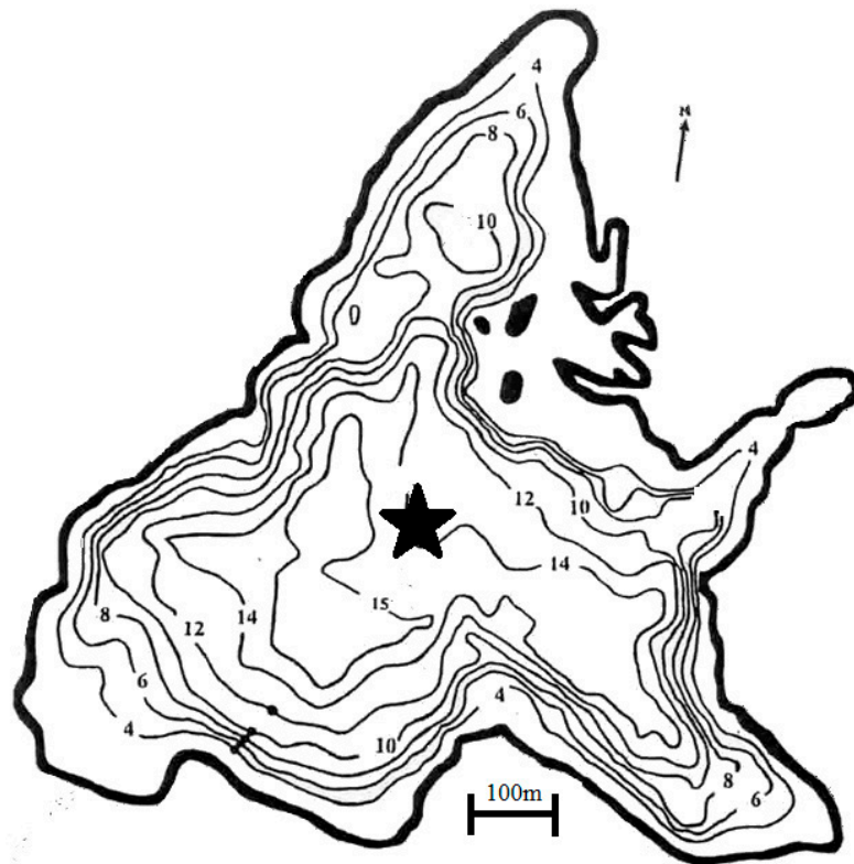
Figure 7. Bathymetric map of Lake Aydat. Star represents the point where the core has sampled.
