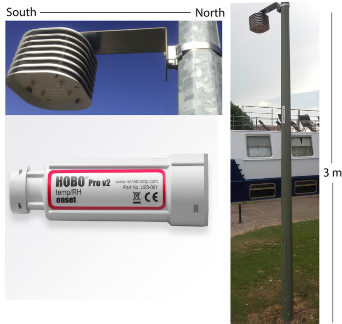
Fig. 6. HOBO U23 Pro v2 sensor, non-aspirated M-RSA Solar Radiation Shield, and a street lamp, with a hose clamp at 3 m above ground.
