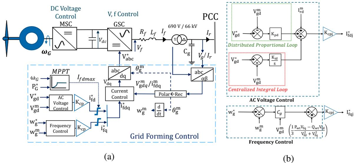
Fig.2: (a) Grid Forming Solution Proposed for Multiple Wind Generators [6] (b) Distributed and Centralized Parts of the Controllers
