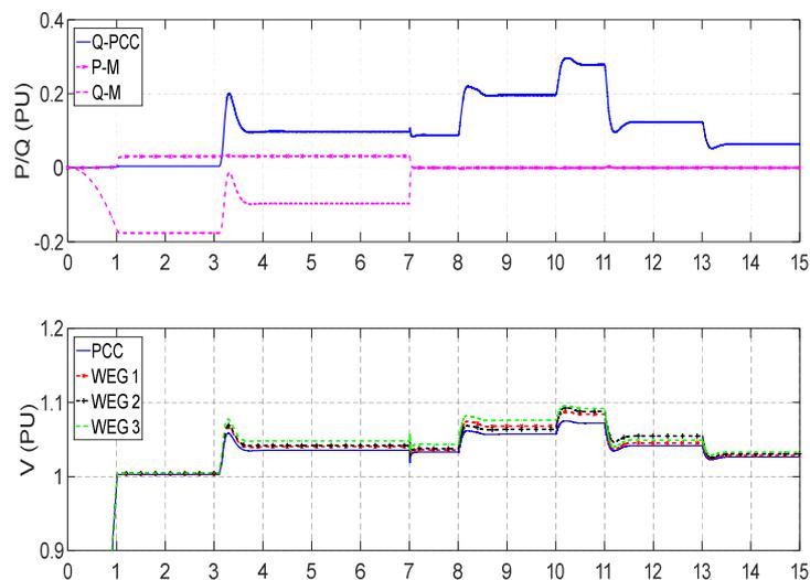
Fig.8: (Top) P, Q injection by the Pseudo Umbilical and Q at PCC; (bottom) RMS AC voltage at various terminals
