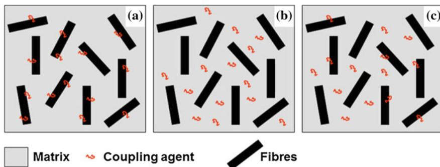
**Fig. 3.7** Possible localization of the coupling agent molecules within the composite microstructure after reactive compounding. **a** All the molecules diffuse at the interface and are grafted on the fibres; **b** all the molecules stay free in the matrix; **c** only a part of the molecules diffuse at the interface and are grafted on the fibres
