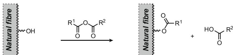
**Fig. 3.1** Esterification reaction of lignocellulosic fibres with anhydride
