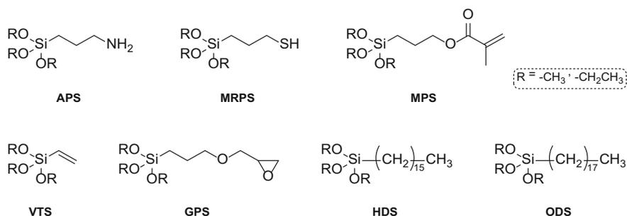
**Fig. 3.3** Chemical structure of various organosilanes. APS:  $\gamma$ -aminopropyl trialkoxy silane; MRPS:  $\gamma$ -mercaptopropyl trialkoxy silane; MPS:  $\gamma$ -methacryloxypropyl trialkoxy silane; VTS: vinyl trialkoxy silane; GPS:  $\gamma$ -glycidylpropyl trialkoxy silane; HDS: hexadecyl trialkoxy silane; ODS: octadecyl trialkoxy silane
