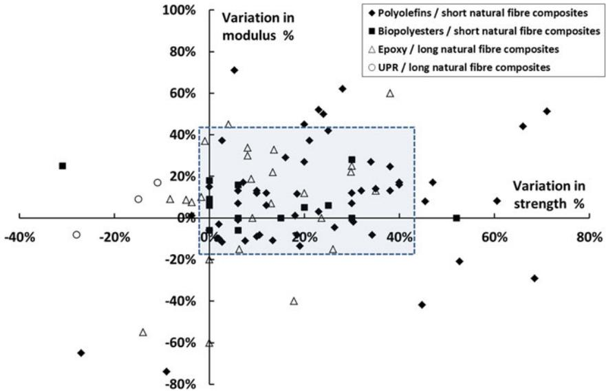
**Fig. 3.8** Ashby plot—variation in modulus versus variation in strength of natural fibre reinforced composites consecutive to pre-treatments and/or functionalization of natural fibres. Non-exhaustive set of data taken from literature for polyolefins and biopolyesters/short fibre composites (tensile properties) and epoxy and unsaturated polyester (UPR) resins/long fibre composites (flexural or tensile properties)
