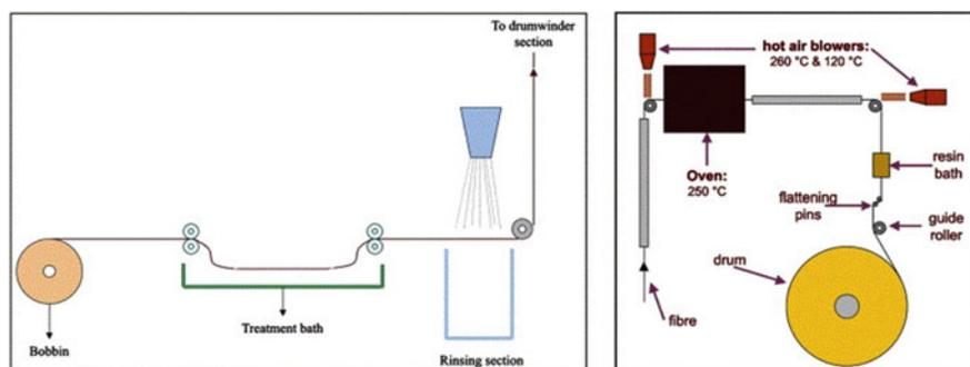
**Fig. 3.4** Sketch of the treatment section and the successive drying section in the fully continuous production set-up. Reprinted from Van de Weyenberg et al. (2006), Fig. 5 with permission from Elsevier
