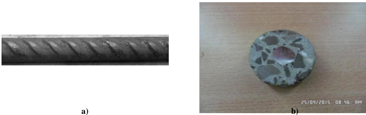
Figure 1: Rebar of steel type BE500S, a) of nominal diameter 16 mm and b) the same bar inserted into a 45 mm diameter concrete matrix used for the interfacial indentation test.
