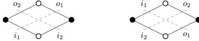
Figure 16: Entries of R(f) (left) and \bar{R}(f) (right) are indexed by the occupation state of (i_1, i_2) and (o_1, o_2) , in the order (absent, absent), (absent, present), (present, absent), (present, present).
