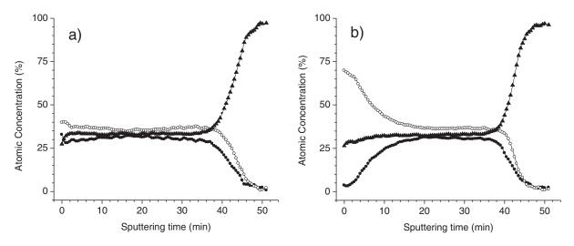
Figure 5. XPS depth profiles of the same k = 2.4 porous dielectric material using identical sputtering rates; a) pristine b) after O<sub>2</sub> plasma treatment. • Carbon,  $\circ$  Oxygen,  $\blacktriangle$  Silicon.
