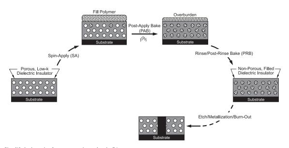
Figure 10. Simplified schematic of process steps integral to the P4 process.
