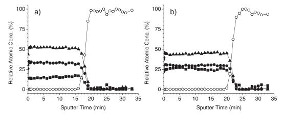
Figure 12. XPS elemental depth profiles of a) unfilled ULK b) ULK refilled with polyacrylate. ■) carbon, ▲) oxygen, ●) ULK silicon, ○) substrate silicon.
