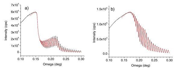
Figure 4. XRR scan and data fitting of a) pristine low-k material, k = 2.2; b) same material after O<sub>2</sub> plasma treatment at 600W for 5sec. — experimental data, — fitted data.
