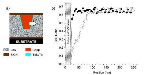
Figure 6. a) Cross-sectional view of TEM-EELS area of analysis (arrow indicates scan direction) and b) C/O elemental ratio as a function of spatial location: • undamaged low-k,  $\circ$  damaged low-k.
