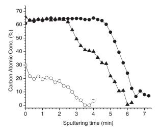
**Figure 11.** Carbon atomic concentration collected by XPS depth-profiling on a dielectric material at k = 1.8 at a fixed filler molecular weight and as a function of fill temperature.  $\circ$ ) unfilled material,  $\blacktriangle$ ) low temperature fill,  $\bullet$ ) high temperature fill.
