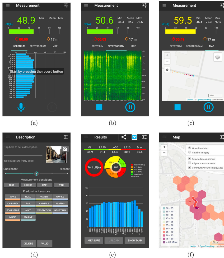
Fig. 1. Screenshots of the NoiseCapture application: (top) ‘Measurement’ views in (a) ‘Spectrum’, (b) ‘Spectrogram’ and (c) ‘Map’ modes; (bottom) (d) ‘Description’, (e) ‘Results’ and (f) ‘Map’ views.
