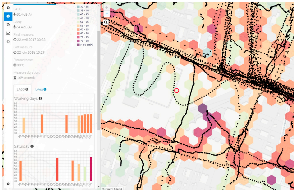
Fig. 5. By selecting an hexagon (from scale factor 16), additional information are given. The location of each measurement point is also available by selecting the corresponding layer. Measurements carried out in the City Center of Lyon (France).
