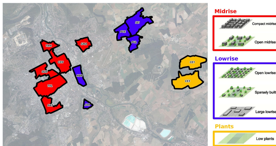
Fig. 11 LCZ groups "Midrise", "Lowrise" and "Plants" based on nocturnal cooling rate values.
