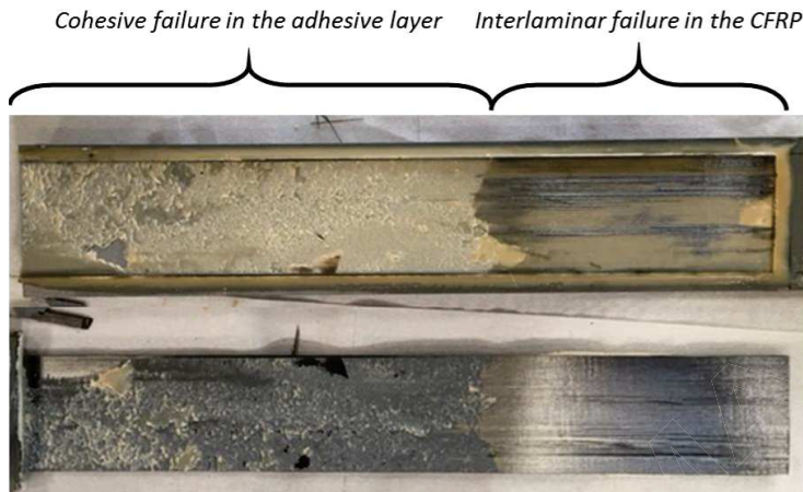
Figure 8: Photo of the observed failure mode (cohesive in the adhesive layer closed to the middle of the sample, and interlaminar in the CFRP plate)
