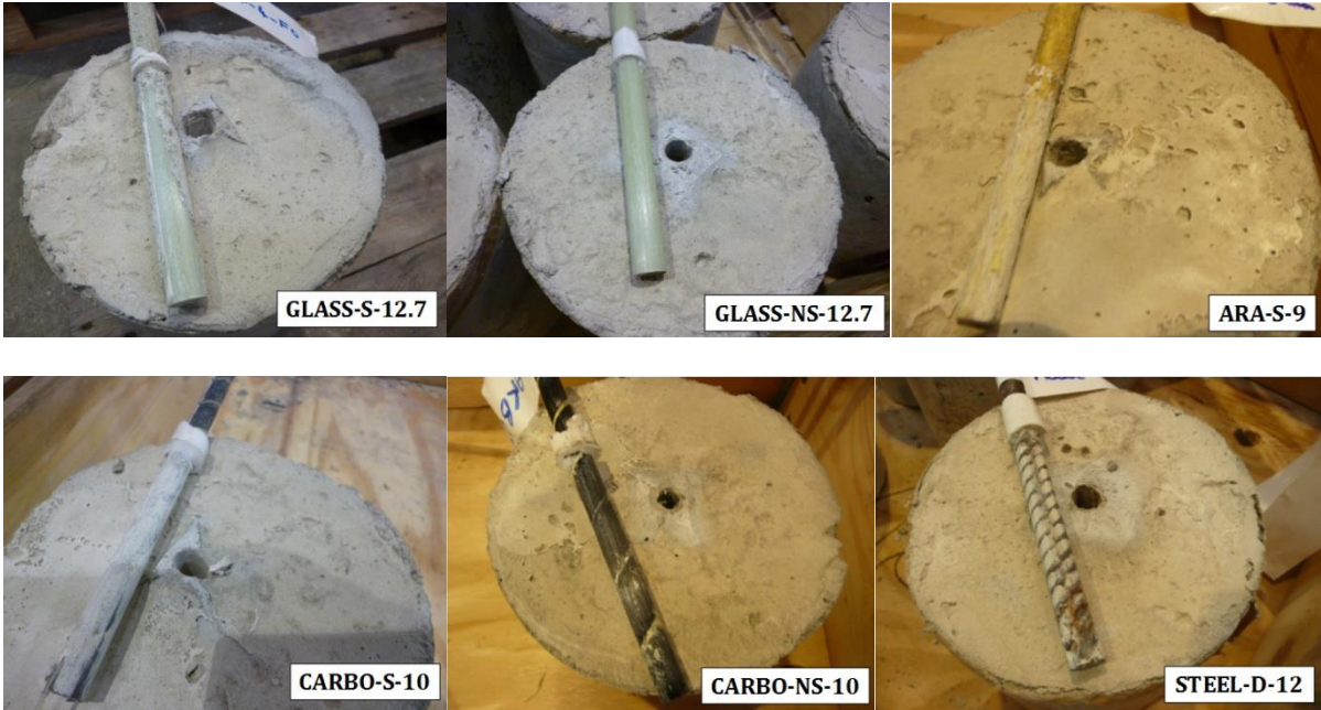
Fig 6. Typical failure modes observed for the various pull-out specimens
