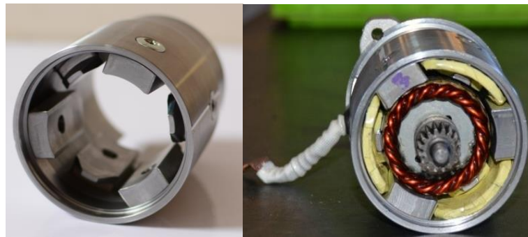
(a) Claw-pole stator armature (b) Whole claw-pole prototype Fig. 11. The claw-pole DC machine manufactured prototype
