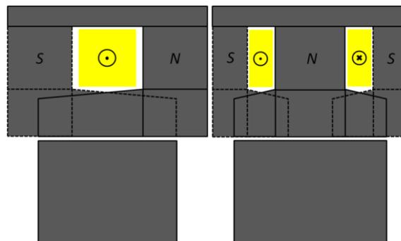
Fig. 3. Single-stack and double-stack stator claw-pole topologies
