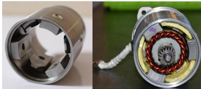
(a) Claw-pole stator armature (b) Whole claw-pole prototype
