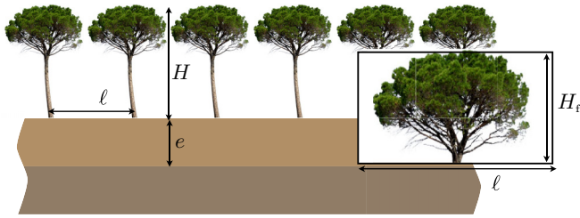
FIG. 1. Periodic array of trees with spacing \ell and total height H ; the ground region is surmounted by a guiding layer able to support Love waves. The tree trunks have a diameter d and filling fraction \varphi_t , and the foliage of height H_f has a surface filling fraction \varphi_f .
