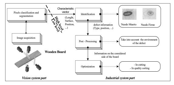
Fig. 3. Functioning principle of the vision system. The part named "low level" deals with the acquisition of the wood board images thanks to the different sensors and the first step of image processing (signal processing). The "high level" part concerns information processing from defect identification to board optimization.
