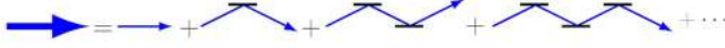
FIG. 2. Schematic of the iterative process expressed by the equation \mathbf{g} = \mathbf{g}^0 + \mathbf{T}\mathbf{g}^0 + \mathbf{TT}\mathbf{g}^0 + \mathbf{TTT}\mathbf{g}^0 + \dots . Each direction change on a wall represents an integral over all the re-emitting walls.
