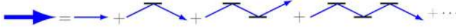
FIG. 2. Schematic of the iterative process expressed by the equation \mathbf{g} = \mathbf{g}^0 + \mathbf{T}\mathbf{g}^0 + \mathbf{T}\mathbf{T}\mathbf{g}^0 + \mathbf{T}\mathbf{T}\mathbf{T}\mathbf{g}^0 + \dots . Each direction change on a wall represents an integral over all the re-emitting walls.
