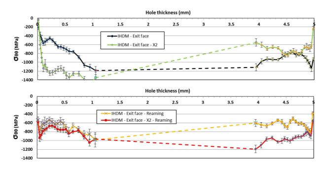
Fig. 9. Stress analysis at the hole edges after cold expansion (top) and after cold expansion and reaming (bottom). Entrance (z=0) and exit face (z=5) measurement connected using
