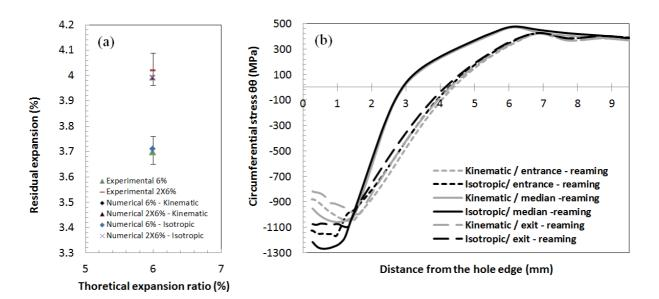
Fig. 11. Analysis of the residual expansion ratio: correlation between experimental and numerical results for single 6% expansion and double successive 6% expansion (a). Scenario
