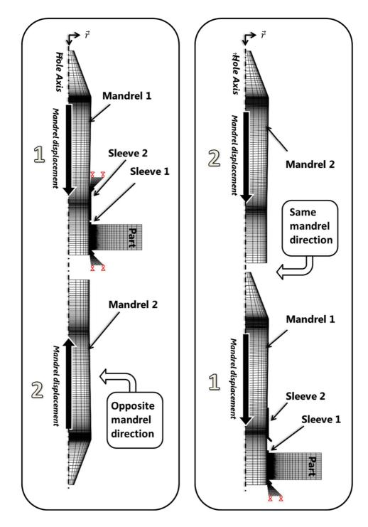
Fig. 1. Axisymmetric modeling of split sleeve expansion process and location of the critical section modeled (taken from a fatigue specimen).
