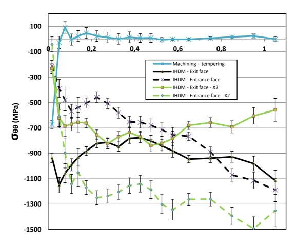
Fig. 7. Stress field measured by IHDM: milled and stress relieved, 6% and  $2 \times 6\%$  in opposite directions, 9.52 mm  $\alpha\beta$  Ti-6Al-4V hole.
