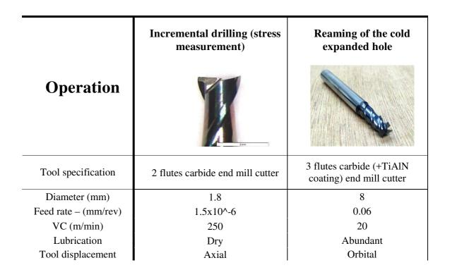
Table. 1. Tools and machining parameters selected for the incremental drilling and reaming
