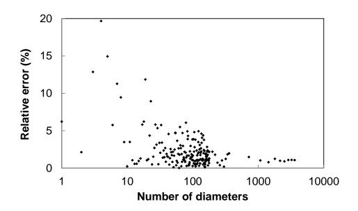
Fig.6. Impact of the number of diameters considered in the diameter algorithm on the relative error of the shrinkage area prediction for the image of calibration
