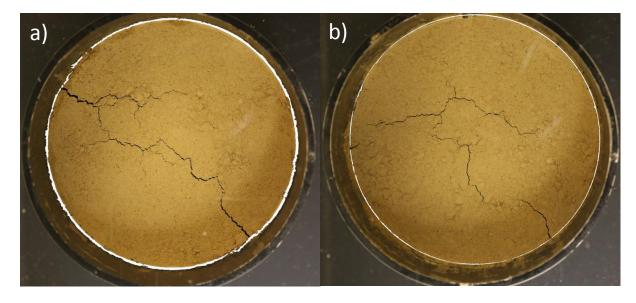
Fig. 2: Image of calibration n°1 after manual determination of the shrinkage area and the crack area (a) and image of calibration n°2 after manual determination of the shrinkage area
