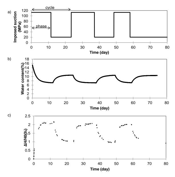
Fig.7. Evolution of the measured parameters over time during the test: a) The imposed suction, b) The specimen water content, c) The vertical shrinkage
