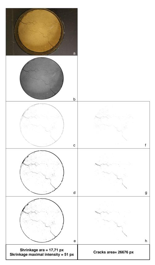
Fig.4. The different stages of the image processing method applied to the calibration image
