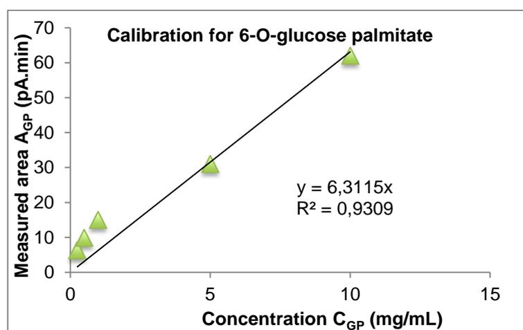
Figure S2: Calibration curve for 6 O-glucose palmitate
