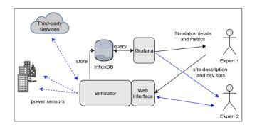
Figure 7: Simulator architecture and use cases
