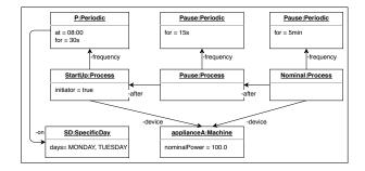
Figure 5: machine behavior modeled with Process
