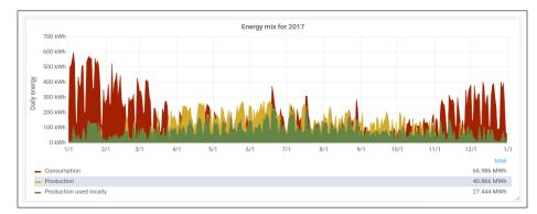
(a) Yearly energy mix of solar production, winter consumption (red) are the most important, due to ventilation and cooling. Most of the production occurs in summer, producing important energy excess (yellow). Here we can see that optimization is required either by reorganizing activities or introducing new type of producer (wind turbine)
