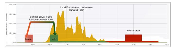
Figure 9: Question 2 : Shifting an activity to a production period when possible increase our self-consumption rate from 9% to 20% for this specific day
