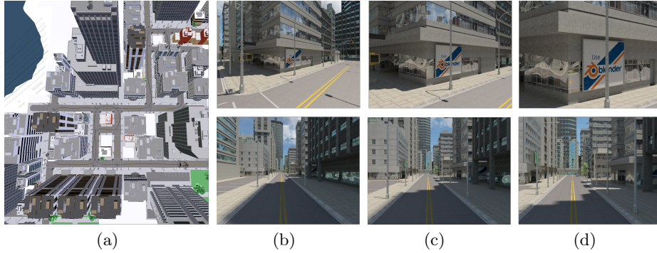
Fig. 4. (a) Top view of the Urban Canyon 3D model. Examples of synthetic images with different fields of view: (b) 80° (c) 60° (d) 40°, each row corresponds to the same camera position.
