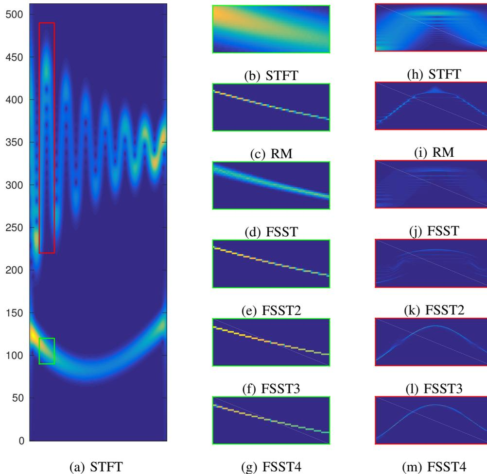
Fig. 3. *Right column panel*, (a): modulus of the STFT of  $f$ . *Middle column panel*, (b): STFT of a small TF patch corresponding to mode  $f_1$  (delimited by green segments) extracted from (a); (c) RM carried out on the STFT shown in (b); from (d) to (g), same as (c) but using respectively FSST, FSST2, FSST3, FSST4. *Left column panel*, same as *middle column panel* but for  $f_2$ .
