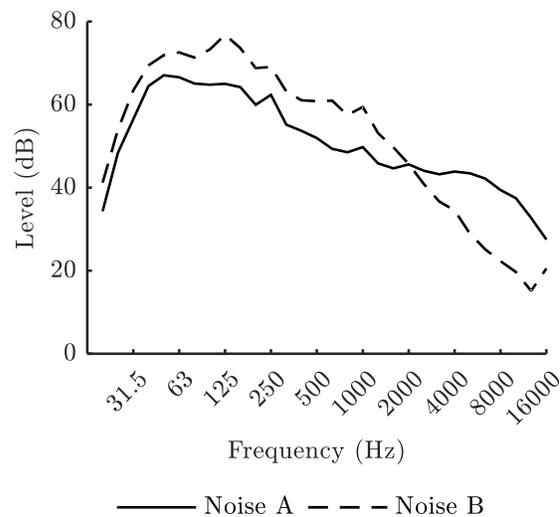
Figure 2: Noise spectra A (50 km/h on a smooth road during a rain shower) and B (130 km/h on a smooth road) recorded in motion at the listener's position.
