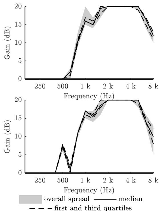
Figure 4: Results of ten repetitions of the genetic algorithm for the search of optimal equalisation values of a speech noise in the maximisation of the SII taking into account a hearing loss level. Top figure: with use of the hearing loss profile P0; bottom figure: with use of the hearing loss profile P1.
