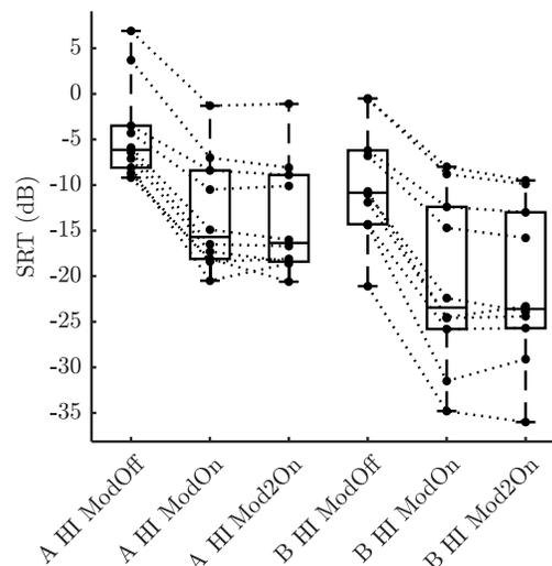
Figure 8: Box and whisker plots and paired comparisons of the effect of speech modifications on the SRT of 10 hearing-impaired subjects. A HI ModOff: test in noise A without speech modifications. A HI ModOn: speech modifications determined from individual hearing loss profiles. A HI ModOn2: speech modifications determined from the averaged hearing loss profile. B HI ModOff, B HI ModOn, B HI ModOn2: same results for noise B.
