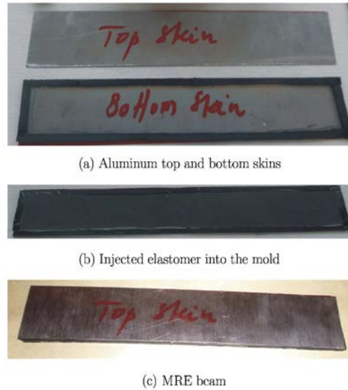
Fig. 5. Steps in fabricating the MRE beam.
