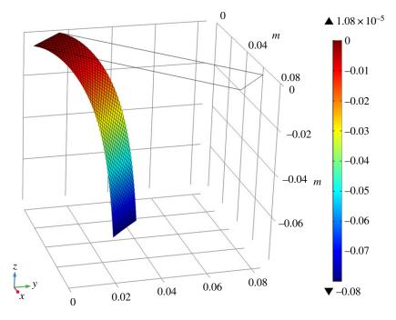
Figure 6. Deformed cantilever strip in bias direction. Colour indicates the out-of-plane displacement. (Online version in colour.)
