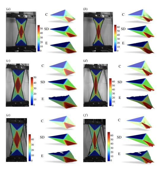
**Figure 7.** UBE test for the samples of size: (*a*), (*b*)  $100 \times 200 \text{ mm}$ ; (*c*), (*d*)  $150 \times 300 \text{ mm}$ ; (*e*), (*f*)  $200 \times 400 \text{ mm}$  (E, experiment; SD, semi-discrete; C, continuum). (*a*) Shear angle approximately  $56^{\circ}$ , (*b*)  $64^{\circ}$ , (*c*)  $50^{\circ}$ , (*d*)  $67^{\circ}$ , (*e*)  $48^{\circ}$  and (*f*)  $68^{\circ}$ . (Online version in colour.)
