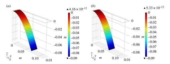
**Figure 3.** Deformed cantilever strip. Colour indicates the out-of-plane displacement. Long fibres along (a) warp and (b) weft directions. (Online version in colour.)
