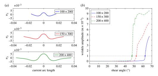
**Figure 9.** UBE test: wrinkling details by semi-discrete model. (a) Out-of-plane displacement along a mid-section for the samples  $100 \times 200$ ,  $150 \times 300$  and  $200 \times 400$  with shear angles  $64^{\circ}$ ,  $67^{\circ}$  and  $68^{\circ}$ , respectively. (b) Post buckling behaviour. (Online version in colour.)
