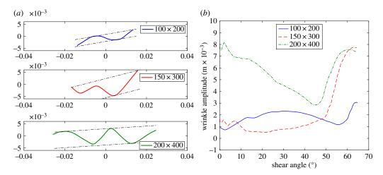
**Figure 10.** UBE test for the three experimental specimens. (a) Profile through mid-section at 63.7°, 68.5° and 67.8° together with two parallel amplitude measurement lines positioned above and below the cross section profile. (b) Amplitude versus shear angle, the wrinkle onset angle is identified by the start of the sharp increase in amplitude apparent at higher shear angles. (Online version in colour.)
