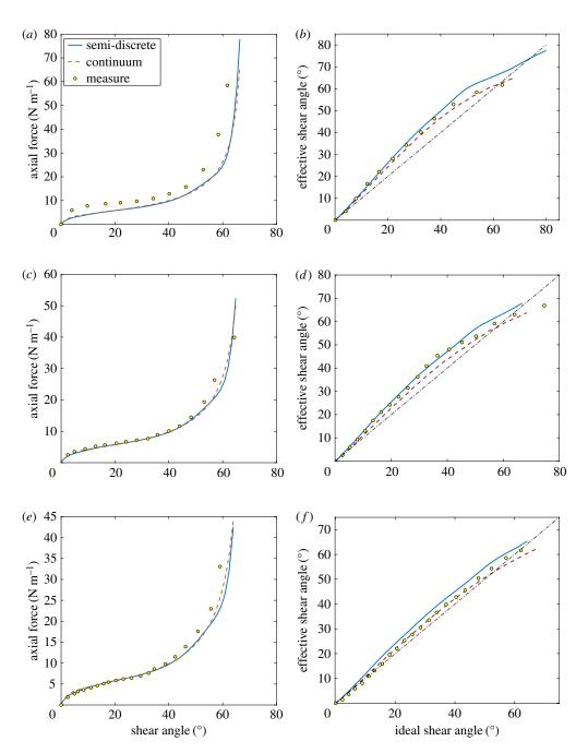
**Figure 4.** UBE test for the samples of size: (a,b) 100  $\times$  200 mm; (c,d) 150  $\times$  300 mm; (e,f) 200  $\times$  400 mm. (a,c,e) Normalized axial force versus shear angle. (b,d,f) Effective shear angle versus ideal shear angle. (Online version in colour.)
