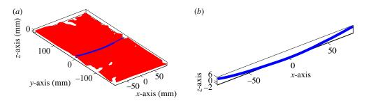
**Figure 11.** Morphology of  $200 \times 400$  mm specimen at the start of the test. (a) Out-of-plane displacement of the whole specimen at the start of the test. (b) The profile of the mid-section cross section of the sample showing about 8 mm of out-of-plane displacement. (Online version in colour.)
