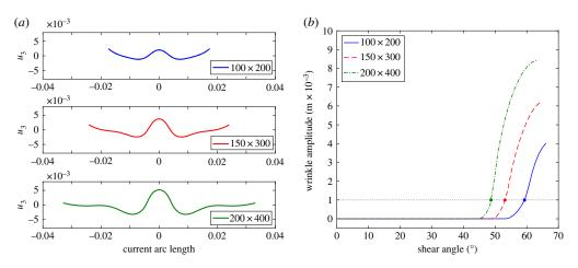
**Figure 8.** UBE test: wrinkling details by continuum model. (*a*) Out-of-plane displacement along a mid-section for the samples  $100 \times 200$ ,  $150 \times 300$  and  $200 \times 400$  with shear angles  $64^{\circ}$ ,  $67^{\circ}$  and  $68^{\circ}$ , respectively. (*b*) post buckling behaviour. (Online version in colour.)
