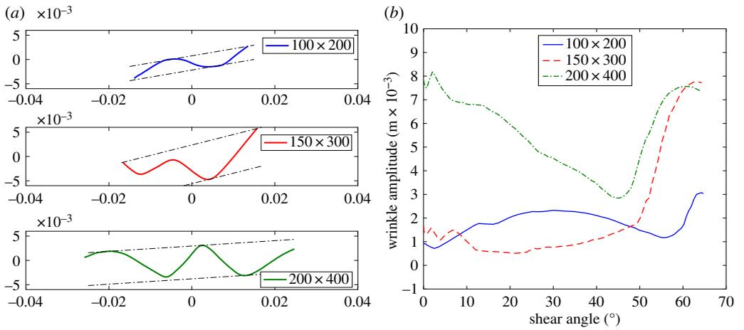
**Figure 10.** UBE test for the three experimental specimens. (a) Profile through mid-section at  $63.7^\circ$ ,  $68.5^\circ$  and  $67.8^\circ$  together with two parallel amplitude measurement lines positioned above and below the cross section profile. (b) Amplitude versus shear angle, the wrinkle onset angle is identified by the start of the sharp increase in amplitude apparent at higher shear angles. (Online version in colour.)
