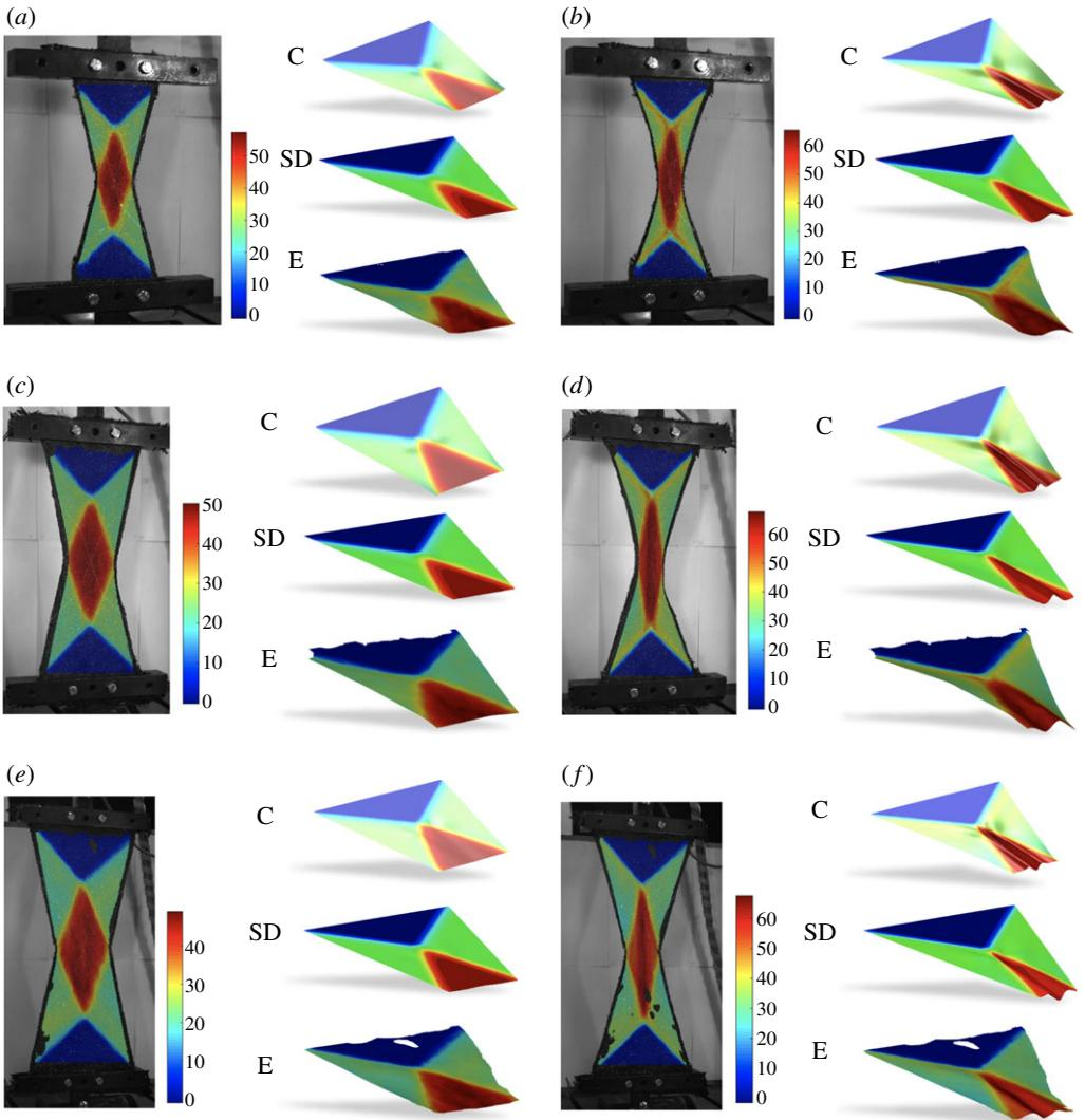
**Figure 7.** UBE test for the samples of size: (a), (b)  $100 \times 200$  mm; (c), (d)  $150 \times 300$  mm; (e), (f)  $200 \times 400$  mm (E, experiment; SD, semi-discrete; C, continuum). (a) Shear angle approximately  $56^\circ$ , (b)  $64^\circ$ , (c)  $50^\circ$ , (d)  $67^\circ$ , (e)  $48^\circ$  and (f)  $68^\circ$ . (Online version in colour.)
