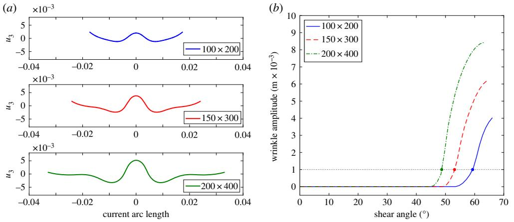
**Figure 8.** UBE test: wrinkling details by continuum model. (a) Out-of-plane displacement along a mid-section for the samples  $100 \times 200$ ,  $150 \times 300$  and  $200 \times 400$  with shear angles  $64^\circ$ ,  $67^\circ$  and  $68^\circ$ , respectively. (b) post buckling behaviour. (Online version in colour.)
