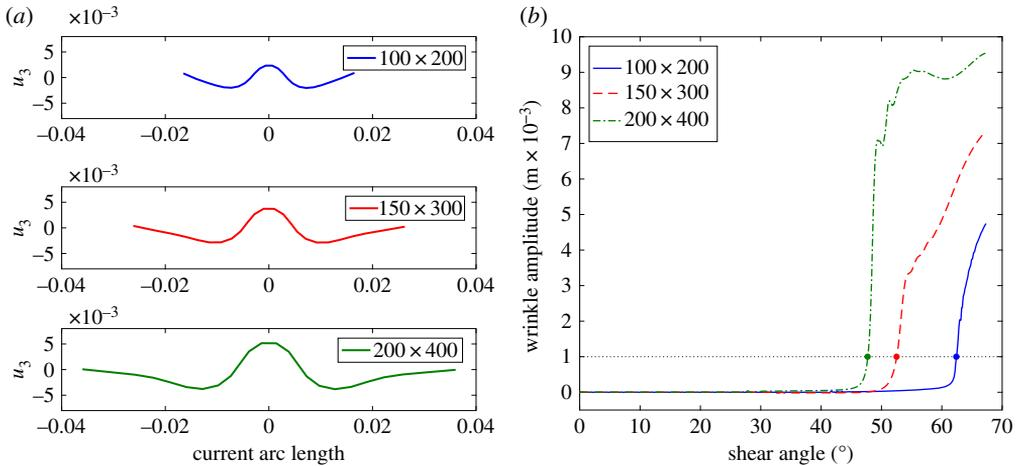
**Figure 9.** UBE test: wrinkling details by semi-discrete model. (a) Out-of-plane displacement along a mid-section for the samples  $100 \times 200$ ,  $150 \times 300$  and  $200 \times 400$  with shear angles  $64^\circ$ ,  $67^\circ$  and  $68^\circ$ , respectively. (b) Post buckling behaviour. (Online version in colour.)
