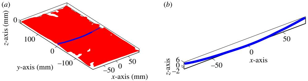
**Figure 11.** Morphology of  $200 \times 400$  mm specimen at the start of the test. (a) Out-of-plane displacement of the whole specimen at the start of the test. (b) The profile of the mid-section cross section of the sample showing about 8 mm of out-of-plane displacement. (Online version in colour.)
