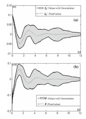
Fig. 8 The behavior of Macpherson suspension system when excited by an instantaneous displacement (response calculated with the use of exponential Horner with reduction). **a** Vertical displacement of mass  $m_s$  calculated by applying Horner exponential with reduction. **b** Rotational movement of mass  $m_s$  calculated by applying Horner exponential with reduction
