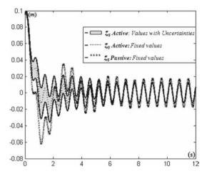
Fig. 12 MacPherson suspension system response when excited with snap-displacement. a Vertical displacement of mass ms calculated by applying Horner exponential with reduction.
