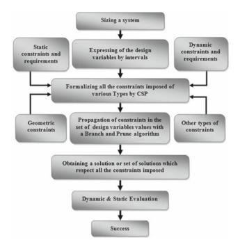
Fig. 2 Interval based design process
