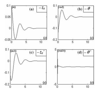
Fig. 6 MacPherson suspension system response when excited with snap-displacement. **a** Vertical displacement of mass  $m_s$ . **b** Rotation of mass  $m_s$  around X. **c** Linear velocity of mass  $m_s$ . **d** Angular velocity of mass  $m_s$
