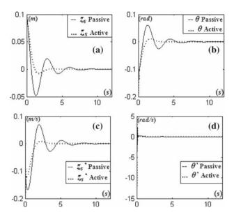
Fig. 10 Comparison between active and passive MacPherson suspension system response when excited with snap-displacement. **a** Vertical displacement of mass  $m_s$ . **b** Rotation of mass  $m_s$  around X. **c** Linear velocity of mass  $m_s$ . **d** Angular velocity of mass  $m_s$
