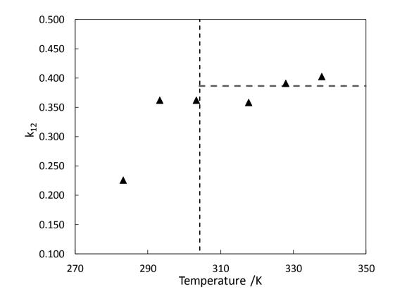
**Figure 5.**  $k_{12}$  binary parameter as a function of temperature. Vertical dashed line: CO<sub>2</sub> critical temperature. Horizontal dashed line: parameter value obtained after considering all the data for  $T > T_c$  (CO<sub>2</sub>).
