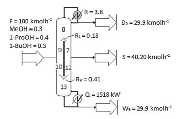
Fig. 6. Structural and operational parameters of DWC system.
