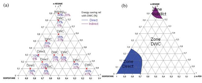
Fig. 16. Energy saving (a) and optimal regions (b) on the composition space for M2.
