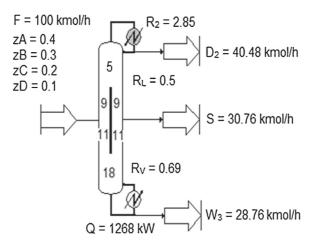
Fig. 8. Design parameters for the divided wall column.
