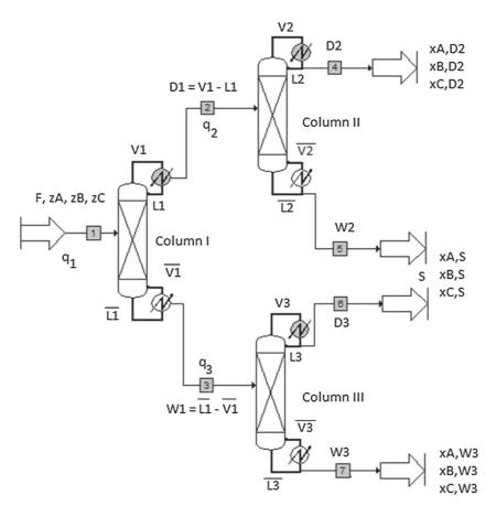
Fig. 2. Simplified model design of divided wall column.
