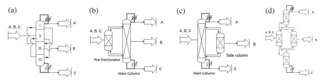
Fig. 3. Models for simulation: (a) pump around sequence (b) two-column sequence with prefractionator (c) two-column sequence with postfractionator (d) four-column sequences.
