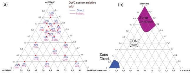
Fig. 14. Energy saving (a) and optimal regions (b) on the composition space for M1.
