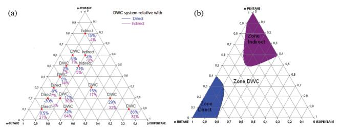
Fig. 15. Energy saving (a) and optimal regions (b) on the composition space for M2.
