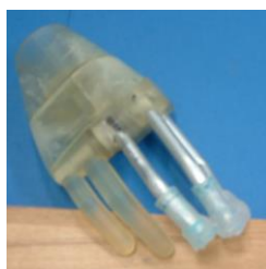
Figure 5 : prototypes de main: a - premier prototype b – second prototype à compliance passive
