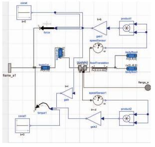
Fig.5. Propeller 1 model implemented in Modelica
