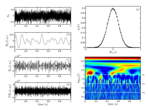
**FIG. 4.** Wavelet-based spectral decomposition of a synthetic fractional Gaussian random signal  $S_d$  with Hőlder exponent h = -0.25, with a Morse wavelet of exponents  $\gamma = 1$ , n = 4. Same representation as in Fig. 3.
