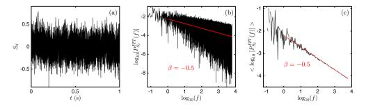
**FIG. 2.** Power spectrum of a fractional Gaussian stochastic signal computed with a standard FFT transform. (a) The signal  $S_d(t)$  (a 1 s portion of this numerical signal of length 80 s) with Hölder exponent h = -0.25. (b) FFT power spectrum. (c) Averaged FFT power spectrum of  $S_d$  on logarithmically distributed frequency values. The total length and sampling time of this numerical signal are identical to the characteristics of the experimental AFM signals investigated in this work.
