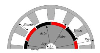
Fig. 3. Prototype SPMSM 12s10p topology description
