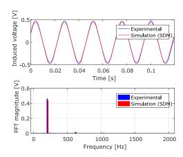
Fig. 6. Induced voltage comparison between SDM and experimentation.
