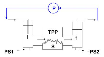
Fig. 10. Sketch of the experimental setup: fracture sample (S), transparent Plexiglas plate (TPP), peristaltic pump (P), pressure sensors (PS1, PS2).
