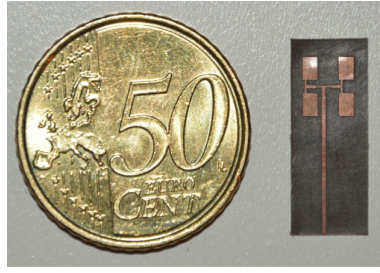
Fig. 1 The 60 GHz four-patch antenna array that is used for the mm-PEM and is denoted as Rx in the text. The antenna is fabricated on an RT Duroid 5880 substrate.
