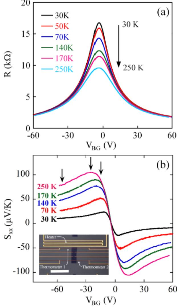
Fig. 2. Thermoelectric measurements in bilayer graphene. (a) Two-terminal resistance  $R$  and (b) thermopower as a function of the backgate voltage  $V_{BG}$  in zero magnetic field and at various temperatures:  $T = 30, 50, 70, 140, 170,$  and  $250$  K. Inset: optical image of a typical device. Size of the scalebar is 30 nm. Reproduced with permission [70]. Copyright 2010, American Physical Society.
