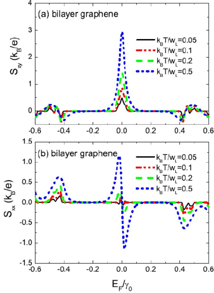
Fig. 4. Thermopower  $S_{xx}$  and Nernst signal  $S_{xy}$  as functions of the Fermi energy in bilayer graphene and at different temperatures. The system size is taken to be  $N = 96 \times 48 \times 2$ , with magnetic flux  $\varphi = 2\pi/48$ , and disorder strength  $r_s = 0.3$  (uniformly distributed positively and negatively charged impurities are considered within this strength) with  $W_{L/\gamma_0} = 0.0376$ . Reproduced with permission [89].
