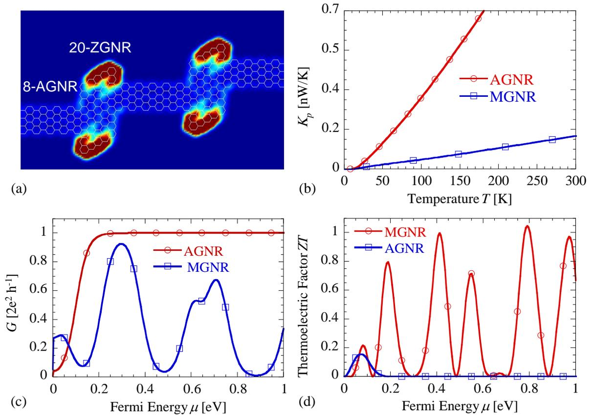
Fig. 5. (a) MGNR consisting of alternating 8-AGNR and 20-ZGNR sections, and local density of states at energy  $E = 0.05$  eV. Red and blue areas correspond to high and low DOS, respectively. (b) Phonon contribution to the thermal conductance as a function of temperature in MGNR and 8-AGNR. (c) Electronic conductance and (d) figure of merit  $ZT$  as a function of chemical potential in both GNRs at room temperature. Further details in Ref. [98].
