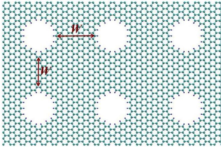
Fig. 9. A typical H-passivated GNM system. Here the big cyan (small blue) spheres represent C (H) atoms, and  $W$  denotes the neck width along the zigzag and armchair directions. Reproduced with permission [147]. Copyright 2012, American Physical Society.
