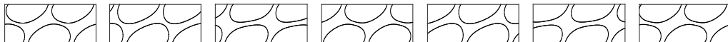
FIGURE 3. Temporal evolution of the bubble configuration for Ca = 0.1 , Bi = 0.1 and Pe = 1 (case B in table 1). Lines corresponds to the liquid-gas interface, i.e. \phi = 0 . The first snapshot corresponds to \tilde{t} = 1.82 and the time interval between two successive snapshots is \Delta\tilde{t} = 0.19 .
