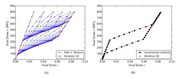
FIGURE 3 – Simulated stress-strain behavior for the case of uniaxial tension.
