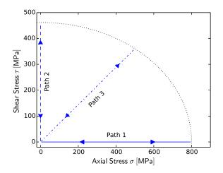
FIGURE 2 – Stress-controlled proportional loading.
