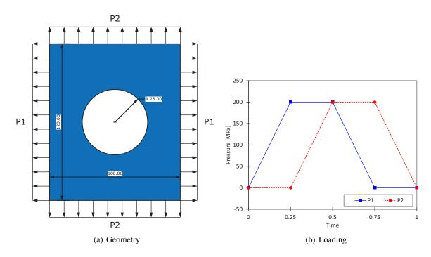
FIGURE 6 – Geometry and loading of a plate with a hole in the center.
