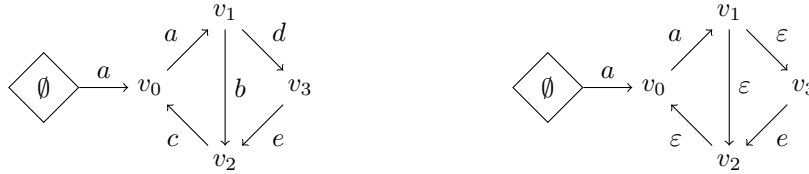
(a) Original control-flow graph for two cache sets: \{a, e\} and \{b, c, d\} .
