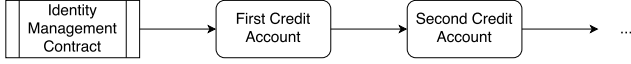
Figure 2. Each credit account is stored in its own instance of the credit account contract. The arrows denote encrypted pointers.
