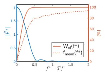
FIG. 1. Spectrum of the dimensionless force (blue). The relative estimation of the radiated elastic energy (red line) and mean frequency (dashed red line) when they are estimated only using the frequency components between 0 and f. They are normalized by the real values computed when the entire spectrum is taken.
