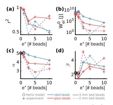
FIG. 13. Scaling law parameters of the elastic energy  $W_{el} = W_{el}^0 R_b^{\alpha} V_b^{\beta}$  fits according to the normalized bed thickness: Rsquare of the fits (a), prefactor  $W_{el}^0$  (b),  $\alpha$  (c), and  $\beta$  (d) coefficients.
