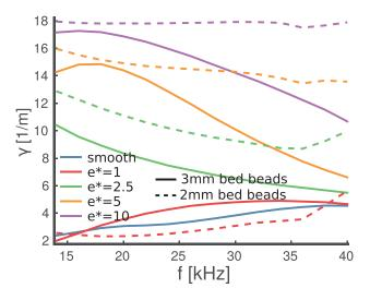
FIG. 5. Viscous attenuation coefficient  $\gamma$  of the PMMA plate for different bed thicknesses  $e^*$  ( $u = u_0/\sqrt{r} \exp\left(-\frac{\gamma}{2}r\right)$ , with *u* the wave amplitude, *r* the source-receiver distance, and  $u_0$  a coefficient).
