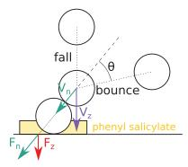
FIG. 11. Picture of the transmission of the force generated by an oblique impact on the rough surface: a bead impacts another one stuck on the plate with an angle  $\theta$ . The normal part  $V_n$  only of the impact velocity  $V_z$  is transferred to the stuck bead and generates a force  $F_n$ . This force is assumed to be totally transmitted to the plate throughout phenyl salicylate. Finally, only the vertical component  $F_z$  of the force F' is measured.
