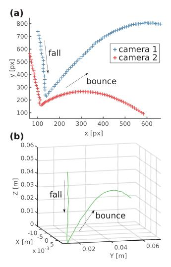
FIG. 7. Stereoscopy processing: combination of two 2D trajectories recorded by 2 fast video cameras (a) in order to obtain the corresponding 3D trajectory (b).
