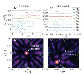
FIG. 6. Localization of the first two impact positions of a 5 mm glass bead on the rough surface using beam-forming with 8 accelerometers. Raw acoustic signals (a) and (b) are back propagated to various test source positions (c) and (d). The color scale corresponds to the criterion  $|\max_t(a_{stack}(t))|$ ,  $*\min_t(a_{stack}(t))|$ ,  $a_{stack}$  being the stack of the 8 back-propagated signals.
