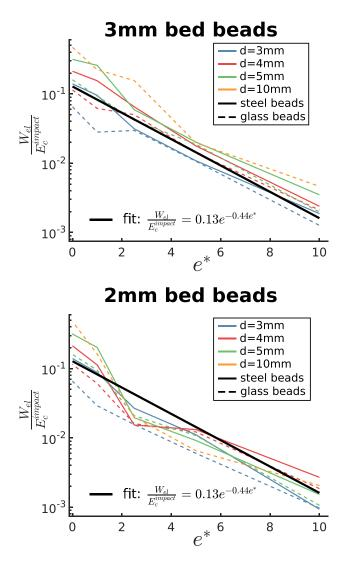
FIG. 9. Ratio between elastic and kinetic energy at the time of impact, as a function of the bed thickness  $e^*$ . Each point corresponds to the average value computed for variable  $V_{z^*}$  sensors, and drop repetitions. The fit is established for all impacts, but impacts on the beds, constituted of 2 mm and 3 mm glass beads, are differentiated for clarity.
