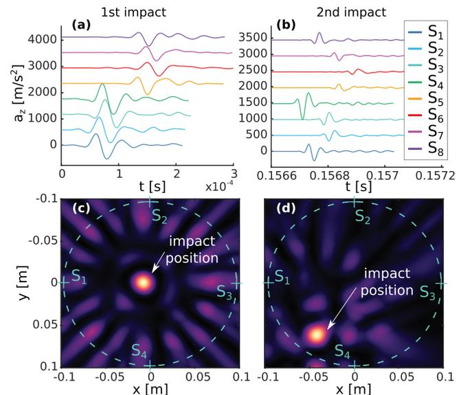
FIG. 6. Localization of the first two impact positions of a 5 mm glass bead on the rough surface using beam-forming with 8 accelerometers. Raw acoustic signals (a) and (b) are back propagated to various test source positions (c) and (d). The color scale corresponds to the criterion  $|\max_t(a_{stack}(t)) * \min_t(a_{stack}(t))|$ ,  $a_{stack}$  being the stack of the 8 back-propagated signals.
