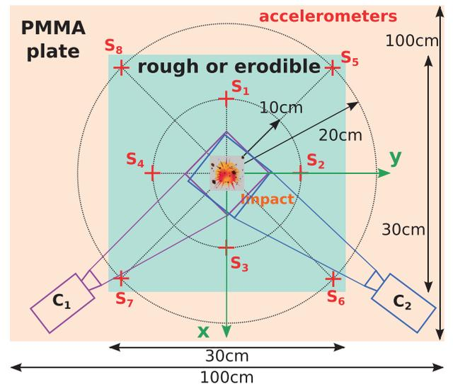
FIG. 3. Sketch of the experimental setup. The red crosses indicate the positions of the sensors  $S_i$ , located at about 10 cm and 20 cm from the impact location. Impacts on the rough surfaces are additionally filmed using two cameras  $C_1$  and  $C_2$ .
