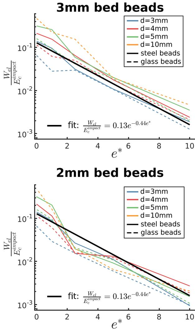
FIG. 9. Ratio between elastic and kinetic energy at the time of impact, as a function of the bed thickness  $e^*$ . Each point corresponds to the average value computed for variable  $V_z$ , sensors, and drop repetitions. The fit is established for all impacts, but impacts on the beds, constituted of 2 mm and 3 mm glass beads, are differentiated for clarity.
