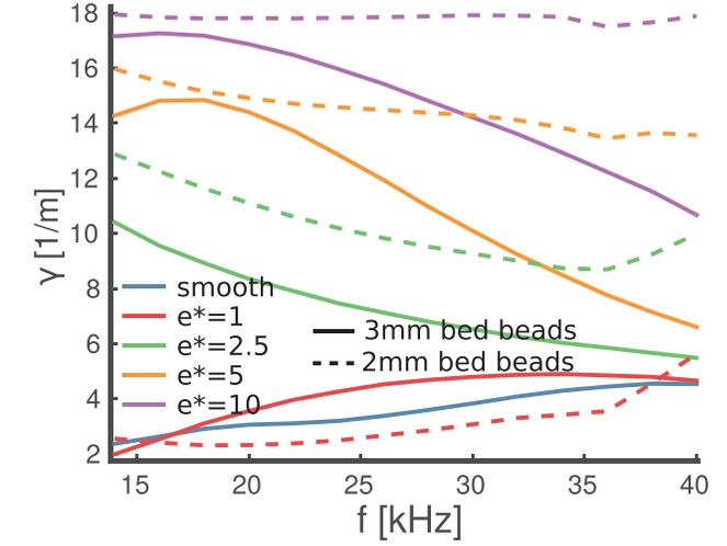
FIG. 5. Viscous attenuation coefficient  $\gamma$  of the PMMA plate for different bed thicknesses  $e^*$  ( $u = u_0/\sqrt{r} \exp(-\frac{\gamma}{2}r)$ , with  $u$  the wave amplitude,  $r$  the source-receiver distance, and  $u_0$  a coefficient).
