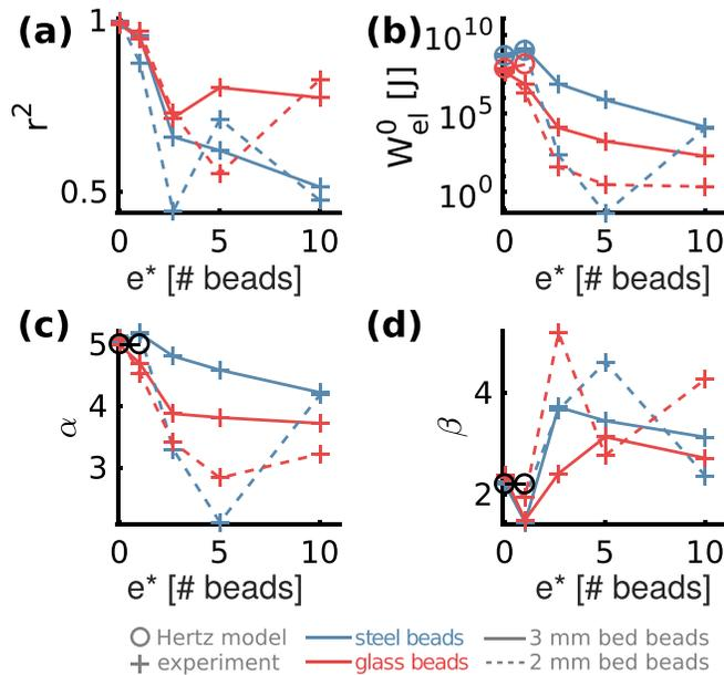
FIG. 13. Scaling law parameters of the elastic energy  $W_{el} = W_{el}^0 R_b^\alpha V_z^\beta$  fits according to the normalized bed thickness: Rsquare of the fits (a), prefactor  $W_{el}^0$  (b),  $\alpha$  (c), and  $\beta$  (d) coefficients.
