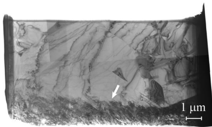
Fig. 2. TEM image of an entire thin foil extracted by FIB from a well recrystallized TiAl sample. The arrow shows a zone containing irradiation damages.
