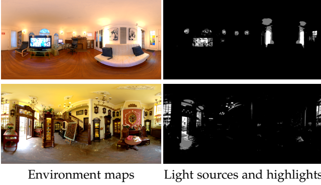
Fig. 6. The detected light sources and highlights of two HDR images. The white areas in the second column indicate the positions of light sources and the grey pixels correspond to highlights.
