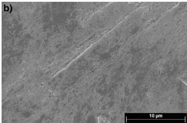
**Fig. 6.** Photograph (A) and SEM micrograph (B) of 1145 carbon steel surface after 24 hour immersion in anaerobic 10 mM phosphate solution pH 7.2 in the presence of 30  $\mu\text{L}$  hydrogenase deactivated by air. SEM characteristics: 10000  $\times$  magnification, 10 kV acceleration voltage.
