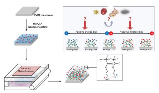
**Fig. 1.** Scheme of research concept of this investigation. Virgin PVDF membranes are coated with TMA and SA monomers, before undergoing plasma polymerization. By carefully choosing the initial monomer ratio, the final surface charge can be controlled. Therefore, it should be possible to regulate the interactions with biofoulants from waters or blood – proteins, bacteria, blood cells, and lead to a low-biofouling surface.
