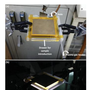
**Fig. 12.** Hand-made glow dielectric barrier discharge plasma treatment. The plasma gas tube feeder and the hole for cooling and air circulation highlighted in (a) are believed to be key engineered parts to optimize in order to improve the final surface homogeneity of surface-modified membranes; (b) Process in operation.
