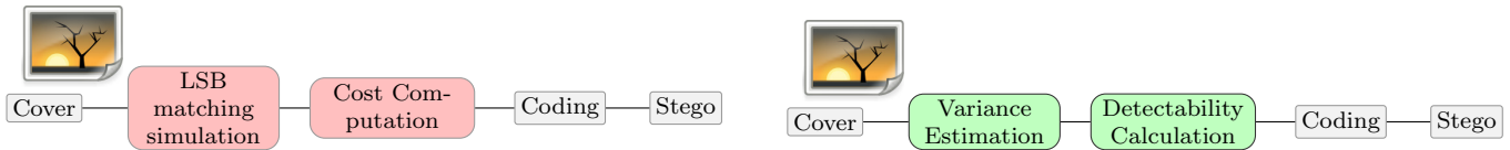
Fig. 1. Simplified flowchart of a typical prior-art adaptive embedding scheme (left) and the proposed MiPOD (right).
