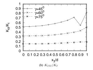
Fig. 6 Stress Intensity Factors for the initial slit
