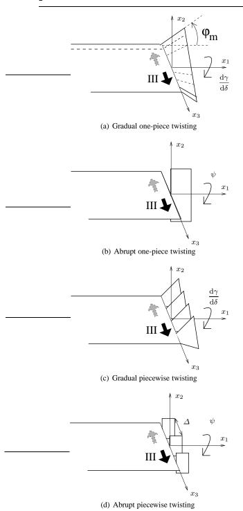
Fig. 1 Several basic propagation possibilities in presence of mode III
