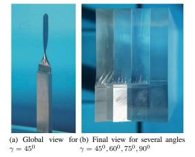
Fig. 3 Gradual one-piece crack twisting
