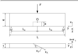
Fig. 2 3PB-specimen with an inclined initial notch
