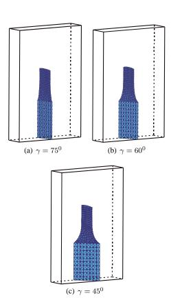
Fig. 9 Computed crack paths
