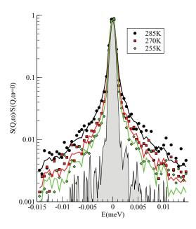
FIG. 2. Quasielastic spectra of PVP/D<sub>2</sub>O sample ( $n_w = 4$ ) obtained by IN16 for  $Q = 1 \text{ Å}^{-1}$  at 285 K, 270 K, and 255 K. Symbols are experimental results, solid lines are fits using a KWW model with  $\beta_{kww} = 0.35$ , convoluted with the measured resolution (indicated in gray).
