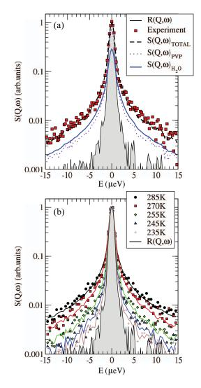
FIG. 4. Quasielastic spectra of PVP/H<sub>2</sub>O sample ( $n_w = 4$ ) at Q = 1 Å<sup>-1</sup> (symbols). Resolution at 2 K is indicated in gray. (a) Results at 270 K. Black dashed line is the total fit, violet dotted line is the polymer contribution and blue solid line is the water contribution. (b) Results at 285 K, 270 K, 255 K, 245 K, and 235 K. Solid lines are fits using two KWW functions or an elastic contribution and a KWW function as described in Eq. (12).
