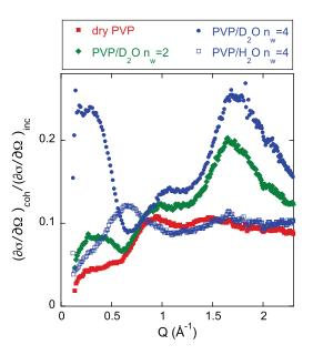
FIG. 1. Ratio between coherent and incoherent differential cross sections for the different samples investigated at RT.
