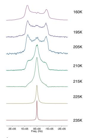
FIG. 9.  $^{2}$ H NMR solid-echo spectra of PVP/D<sub>2</sub>O recorded using a solid-echo delay of 20  $\mu$ s.
