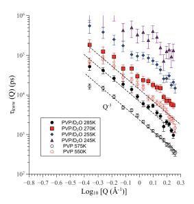
FIG. 3. *Q*-dependence of the relaxation times of dry PVP at 575 K (empty black circles) and 550 K (empty red circles) and PVP in PVP/D<sub>2</sub>O solution ( $n_w = 4$ ) at 285 K (full black circles), 270 K (full red squares), 255 K (full blue diamonds), and 245 K (full black triangles). Dashed lines show a  $\tau_{kww} \propto Q^{-3}$  behavior.
