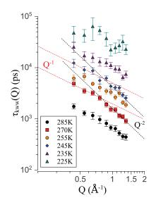
FIG. 5. Relaxation times of water in PVP/H<sub>2</sub>O solution ( $n_w = 4$ ) at different temperatures as function of Q. For Q > 0.7 Å<sup>-1</sup>, the Q-dependence it is compatible with a  $\tau_{kww}^{water} \propto Q^{-2}$  power law, while below it approaches a  $\tau_{kww}^{water} \propto Q^{-1}$  dependence.
